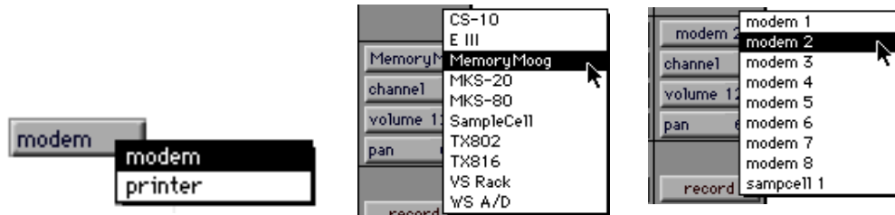
The MIDI Port selector, as it appears without OMS (left) with OMS (center) and with a MIDI Time Piece™ MIDI Interface without OMS (right)
