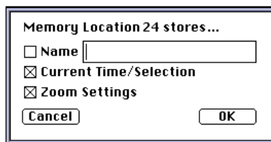
Double-clicking an autolocate button brings up this dialog in which the autolocate point's parameters can be defined.
