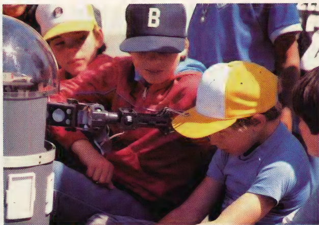
The robot featured a programmable arm that could lift light objects.
