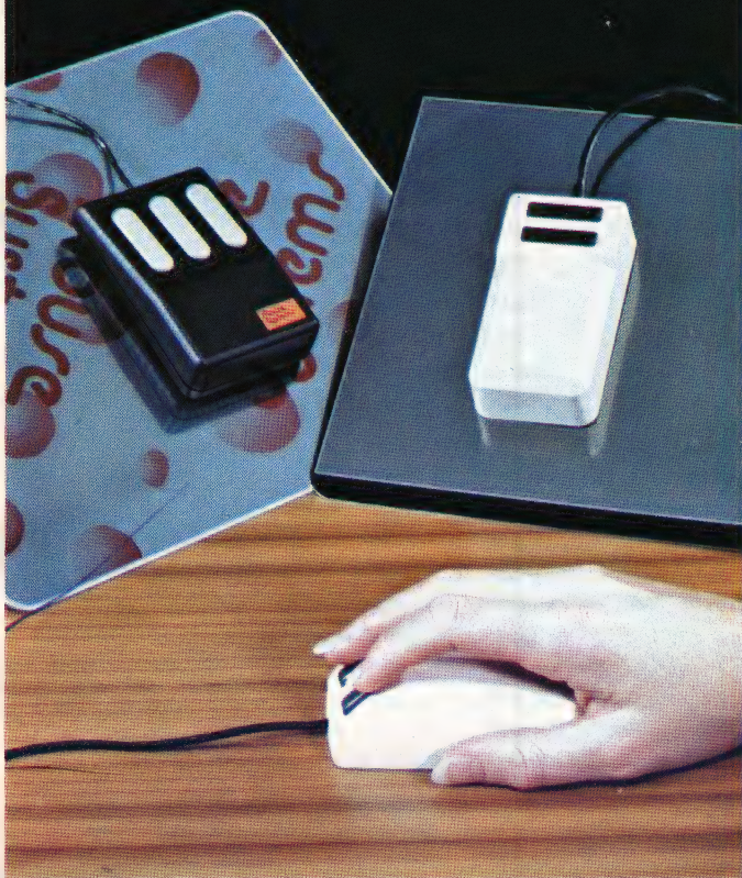
Clockwise from upper left: Mouse Systems and VisuAll's mice both run on their own grids; Microsoft's mouse runs free.
