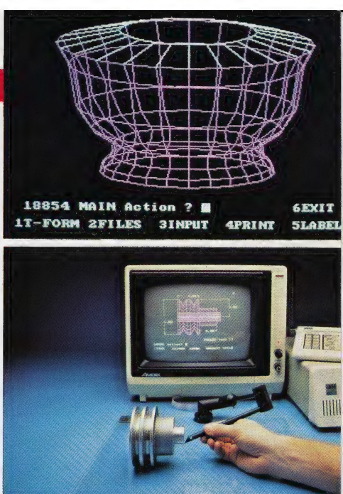
Advanced Space Graphics produces three-dimensional representations of objects, real or imagined. Below, a stylus traces the shape of the object while the screen shows what the computer has seen so far.
