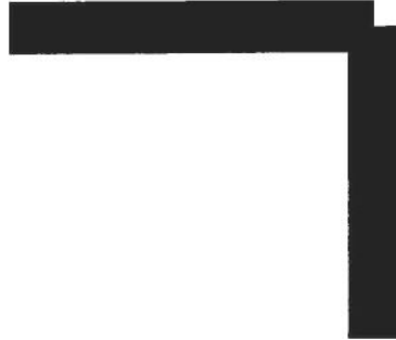
Fig. 4-10: Lines With Butt End Caps
