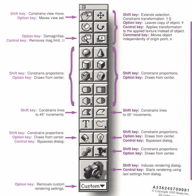
† Shift key constrains rotation on handle rotations only.
