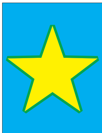
Tint Reduction value of 100%: The resulting trap line contains 100% of the CMYK values of the lighter color
