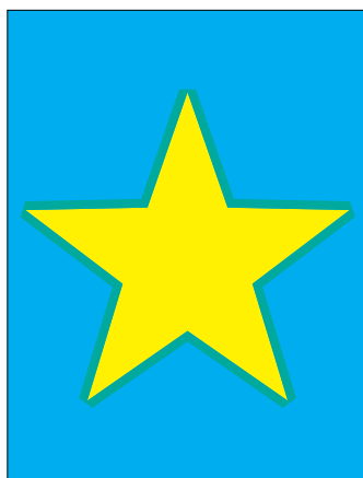
Tint Reduction value of 50%: The resulting trap line contains 50% of the CMYK values of the lighter color
