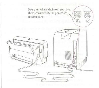
$\triangle$  **Important:** It's OK to connect the StyleWriter II to either the printer port or the modem port.  $\triangle$
