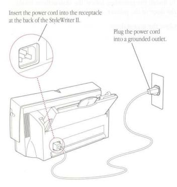
**Warning:** This equipment is meant to be electrically grounded. Do not defeat the purpose of the grounding plug! The StyleWriter II is equipped with a three-wire grounding plug—a plug that has a third (grounding) pin. This plug fits only a grounding-type AC outlet. If you are unable to insert the plug into an outlet, contact a licensed electrician to replace the outlet with a properly grounded one.
