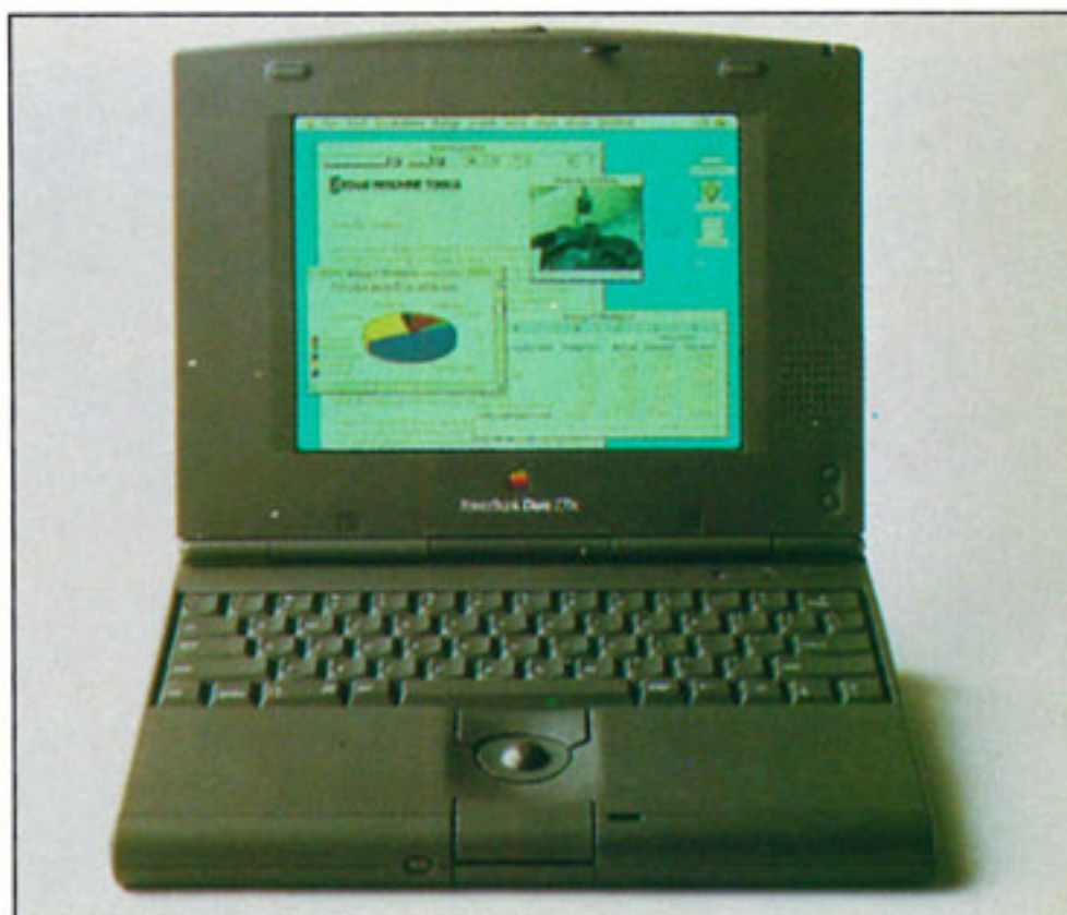
The PowerBook 270c: the first 16-bit colour notebook. It boasts 33MHz, a floating point unit and a rather generous 240Mb hard drive. Existing owners can upgrade their screen to a colour one.
