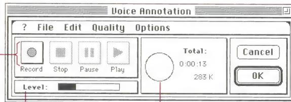
The level meter indicates the volume of the sound.
