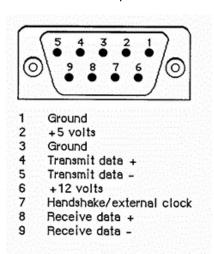
Figure 3. Pinout for SCC Output Jacks
