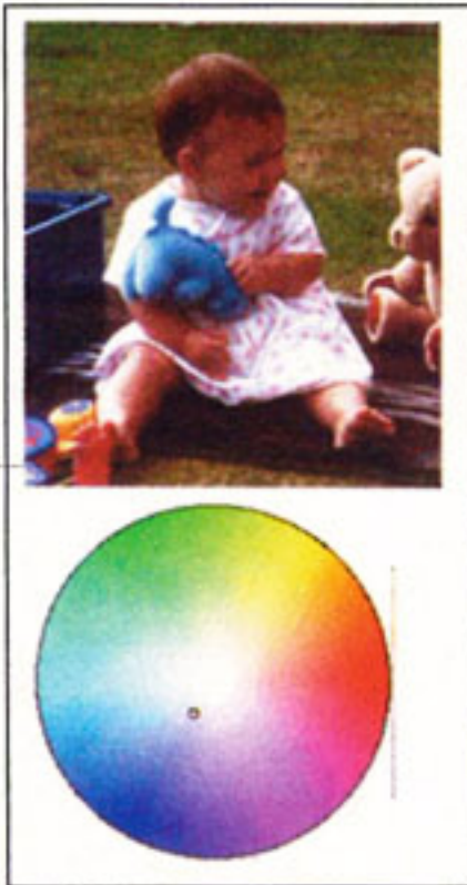
The DeskWriter 310 prints most colours fairly well, if rather pale, but the black is an unpleasant dark olive.
