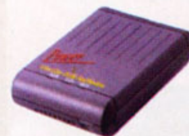
External Fax/Data Modem Physical size : 25mmx105mmx70mm
