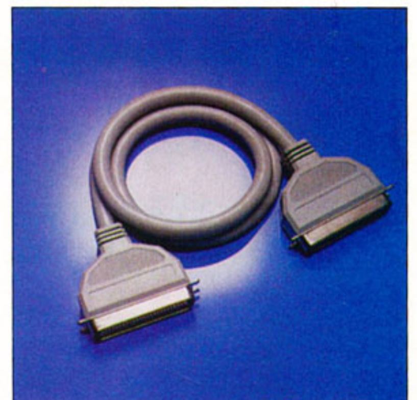
... but you can't connect two SCSI devices together with it – you'll need one like this instead.
