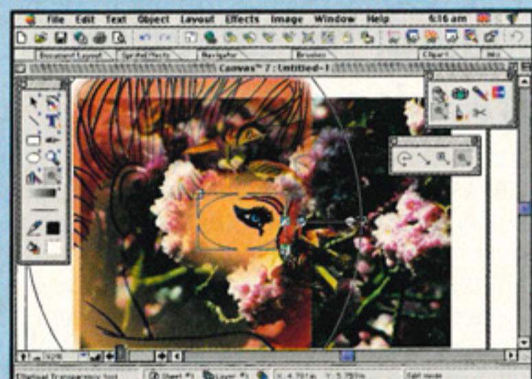
Transparency can be applied in radial, directional, rectangular and elliptical gradients and adjusted manually with on-screen nodes.
