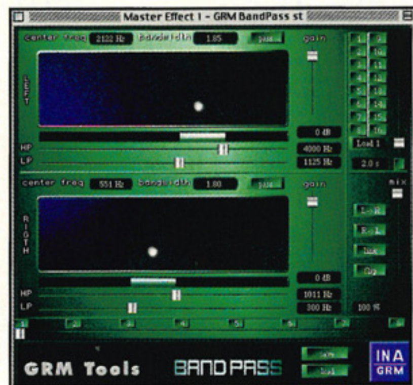
The stereo Band Pass effect can process the left and right channels in different ways.
