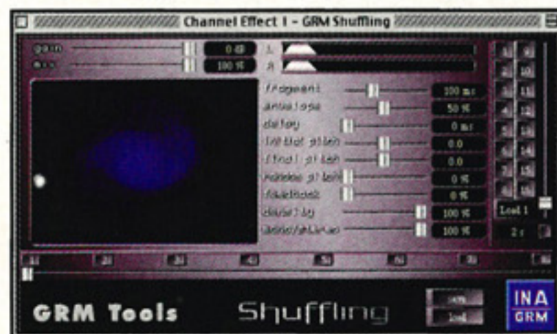
Shuffling cuts the audio into micro-slices and stitches it back together again in a slightly different way.
