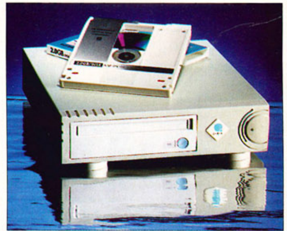
The latest 5.25-inch optical drives can store up to 2Gb of data on to a disk, but will set you back at least £3000.
