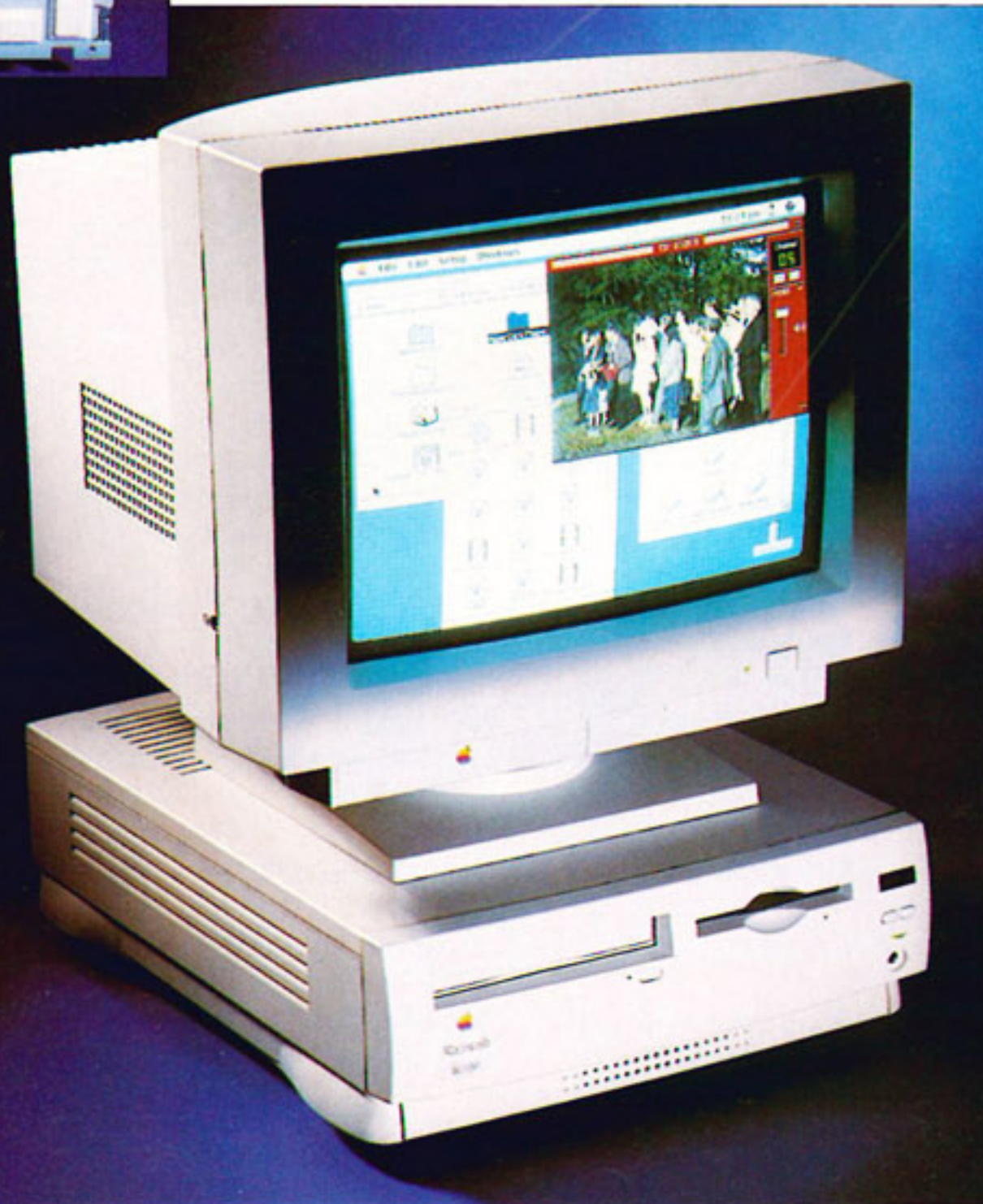
With a Video-In card you can input an S-VHS or Composite signal from a TV, VCR or camcorder, and you can capture this to hard disk at 15 frames per second.
