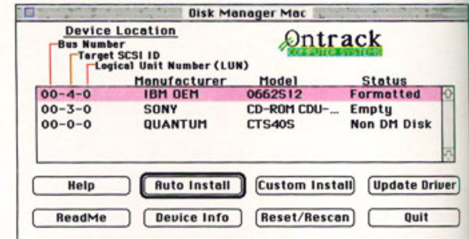
To reformat your hard disk you can use Apple HD SC Setup on the Disk Tools floppy or a commercial program such as Disk Manager Mac (see the review in MACFORMAT 18 ).
