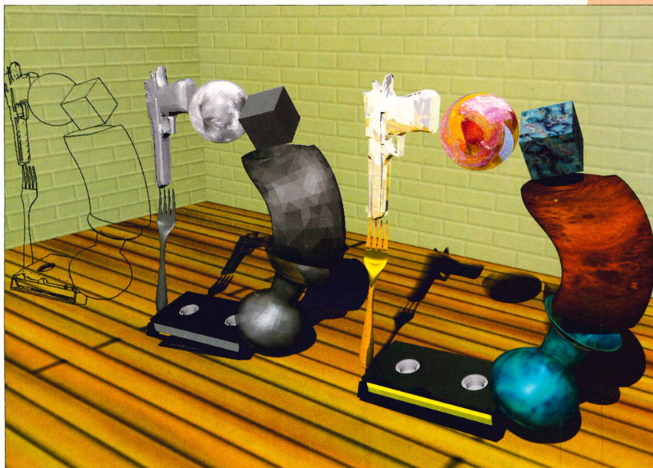
3D programs will render your images in different ways: as wireframes, with hidden line removal for speed (left); as simple faceted objects to show shading and form (centre); and with full photo-realistic 'ray-tracing' for final display versions (right).
